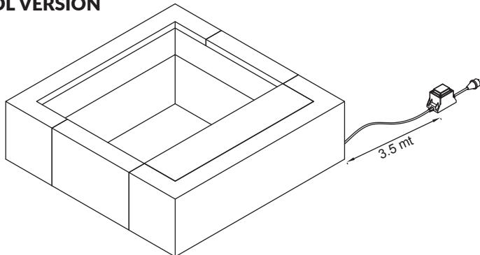
The mini-pool version is the only PLAYA equipped with a special electrical transformer with removable outlet.
