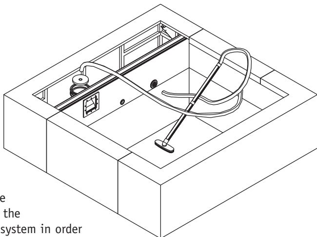
Insert the end of the flexible hose filled with water into the hole on the plate taking care to lift as little as possible.
